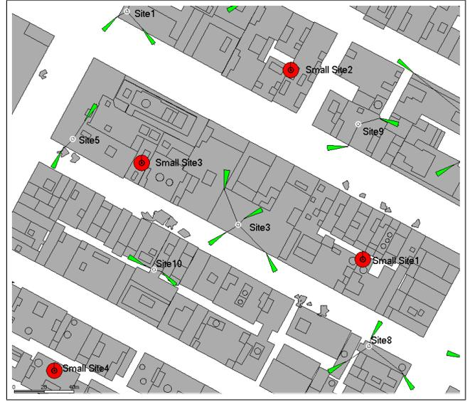
Fig. 2: Network layout showing sites deployment.
