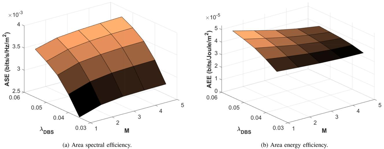
Fig. 10. Performance comparison of CoMP-enabled UCRAN with dynamic blockages with varying DBS densities and  $M$  for  $\gamma_{th} = 4$  dB,  $R_{szone} = 6m$ ,  $\alpha_{near} = 3$  and  $\alpha_{far} = 6$ .
