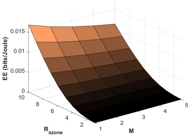
Fig. 7. Energy efficiency of the CoMP-enabled UCRAN with varying S-zone radius and  $M$  for  $\gamma_{th} = 4$  dB.
