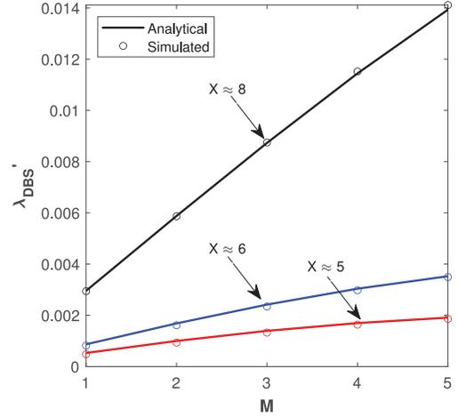
Fig. 3. Average activated DBS density ( $\lambda'_{DBS}$ ) in the network for different numbers of maximum cooperating DBSs ( $M$ ) within an S-Zone.
