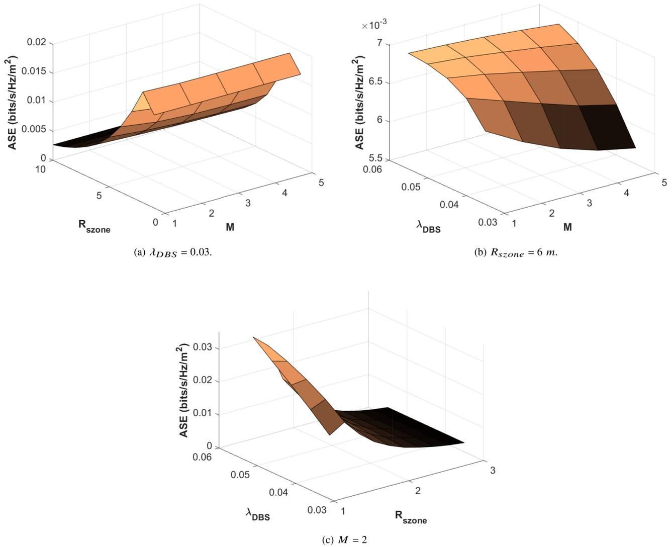
Fig. 6. Area spectral efficiency of the CoMP-enabled UCRAN with varying S-zone radius, DBS density and  $M$  for  $\gamma_{th} = 4 \text{ dB}$ .
