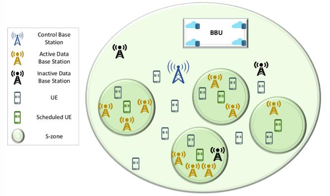
Fig. 1. CoMP-enabled UCRAN architecture with activation region of radius  $R_{szone}$  for a scheduled UE.
